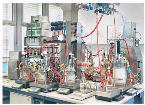
Fig. 1: Multi-bioreactor DoE-plant with BIOSTAT® Bplus and Qplus
